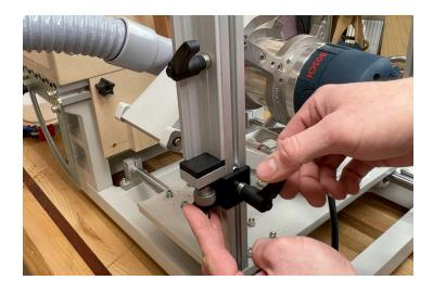
Start by sliding it up until it contacts the bottom of the Template Holder Slider and lock it into position.
