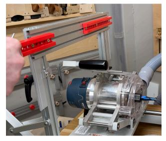
The dado needs to be 3/4" wide, but since it is being cut across the grain, we elected to use our 1/2" Amana spiral up-cut bit rather than a 3/4" straight bit like the one provided in our Monster mortise and tenon set. This means the cut will be made in multiple passes and we will adjust the height of the template holder to get a perfect fit.
