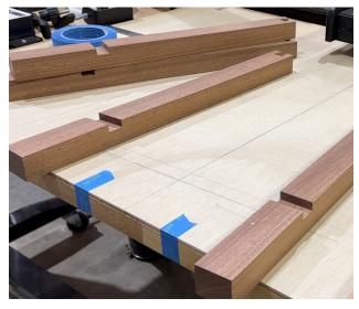
We have been working on a small bench project in the shop and we needed to cut angled slots or dados in the legs to accept the lower shelf. This is a great application for the slot mortising template with some help from our new Template Holder Micro-Adjust.
