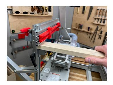
Using the same bit and guide bearing combinations as the standard mortise and tenon templates, for the 1/2" tenon switch to a 22mm guide bearing. Use the outside of the Slot Mortise Template to cut the tenons, starting at the top of the taper.
