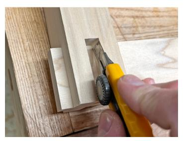
Dry-fit a rail in one of the leg mortises and use a marking knife to locate the location where the intersecting mortise lands on the tenon. Use a square to carry the scribe lines to the bottom edge of the tenon once the joint is disassembled.
