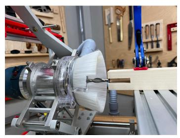
With the Slot Mortise Template stops set so the bit can completely clear either side of the workpiece, cut the first mortise in the end of the leg by incrementally plunging in while moving the router across the template taking small passes at a time.
