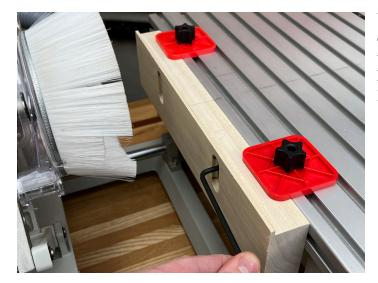
Use the Front Fence Stops overhanging the front edge of the table to position the workpiece support flush with the top table surface and secure it in place using T-Slot hardware from the PantoRouter® Hold-Down Hardware Pack.
