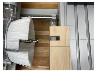
Next, the rails require a notch cut in each tenon to accommodate the intersecting tenon. Since the depth of cut needs to be at least 50% of the tenon height, we need some sort of sacrificial work holding piece on the front of the table to support the workpiece for this operation.
