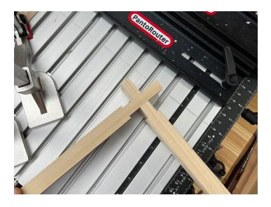
With notches cut on two rails, dry fit the rails and test the fit to confirm the notch is deep enough. The rails should be flush on the top and bottom.
