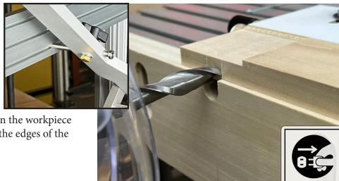
The Auxiliary Fence can be placed against the Centering scale fence to reach far enough forward to register against the end of the rail for repeatable cuts.
