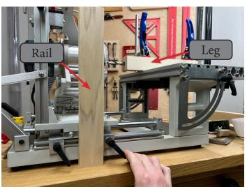
Locate the leg workpiece roughly at the center point of the table, it does not have to be precisely centered since the bit will exit the workpiece on either side of the leg when the mortises are cut. Then set the Centering Scale Fence and clamp the leg down. Use the swing stop to locate the workpiece overhanging the front of the table repeatably.
