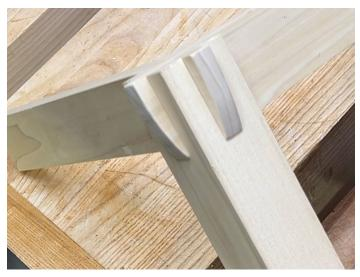
Castle Joints are a great exposed joinery option where a two rails meet at a 90 degree angle with a leg. They are often used on table bases and beds to add a decorative detail and provide a strong joint where multiple piece meet. The components can be glued together for a strong permanent joint or this could be a knock-down joint with optional wedges, hardware, or dowels to lock it into place.
