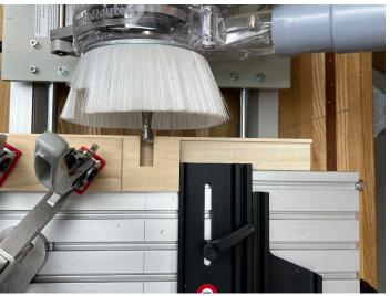
Use the B-V template centered on the template holder and set the Template holder height so the router bit can clear the top and bottom of the tenon. The D-V template can be used for thicker workpieces. Set the depth of cut to be at least 50% of the tenon height and cut the 1/2" notch.
