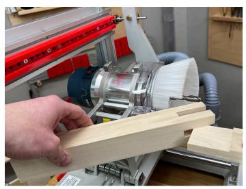
Cut the tenon on the end of the rail workpiece and use the mortise in the leg to test the fit. Use the outside taper on the template to dial in the desired fit depending on if it will be a glue joint or knock-down joint.
